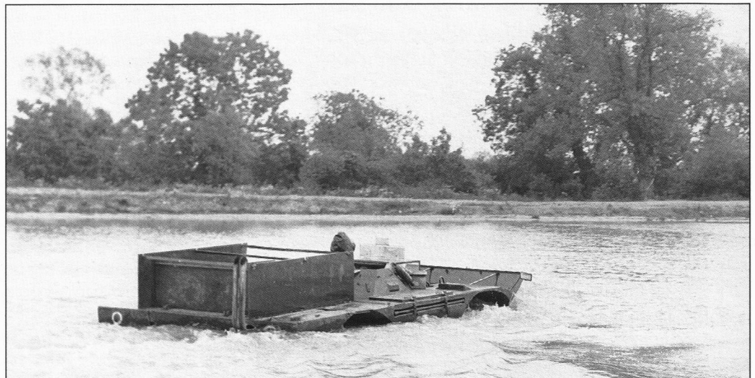
Centre right. This is a Mk 2/3 rigged for amphibious trials by the use of rubberised flotation bags. A metal screen erected around the engine compartment covers helped to prevent the vehicle becoming unstable due to gross leakage at the rear. (TMB, 2802 A3)
