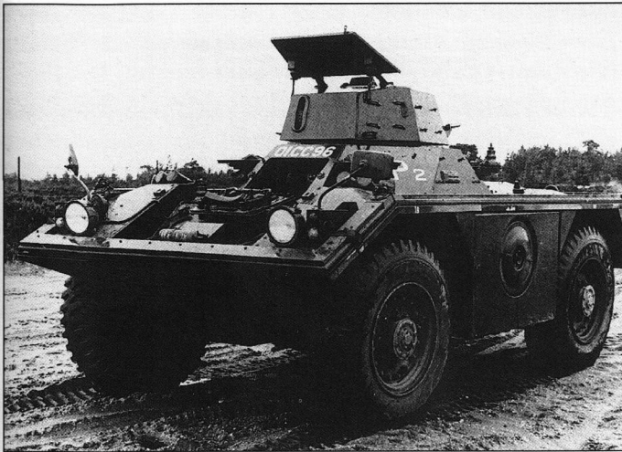
Above. Second prototype of the Mk 4 variant undergoing trials at FVRDE. This example was converted from a Mk 2/3 probably dating from around 1958. (TMB, 2058 D3)
